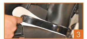
Release the two Tekna<sup>®</sup> lock screws on the gullet plate with the allen key provided.
